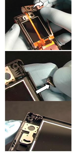
If the volume key fell out, make sure its spring is still attached. Then place it back into its slot in the back cover with the spring facing downward into the back cover.
