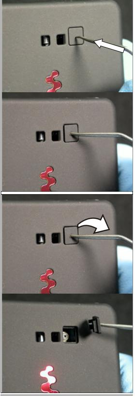
Rotate the dental hook to get the RF port plug to lift out of its opening in the back cover.
