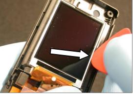
Insert the corner of a plectrum in the seam along one side of the LCD in the location shown.
