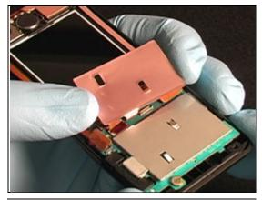
Use the flat end of a nylon pointer to push the LCD flex film out of its connector toward the LCD.
