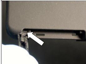
Insert the RF port plug in the opening in the new back cover and press it into place.
