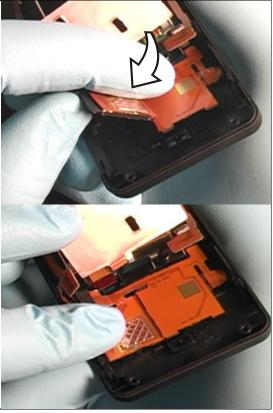
Position the backup battery portion of the SIM flex within its alignment features on the back cover.
