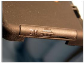
Press the memory stick cover's tab into its hole in the new back cover. Use a nylon pointer if needed.
