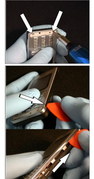
Insert the tip of a plectrum in the seam between the front and back covers in the location shown.
