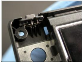
Obtain a new volume key and make sure its spring is correctly attached.
