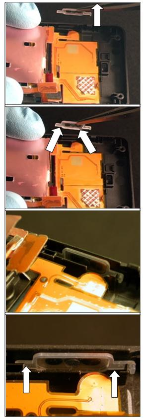
Obtain a new camera key and orient it so that the two curved corners indicated are towards the back cover.
