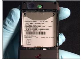
WHEN INSTALLING A NEW LABEL, BE VERY CAREFUL TO AVOID TOUCHING THE CONTACTS OF THE BATTERY CONNECTOR WITH THE ADHESIVE SIDE OF THE LABEL.
