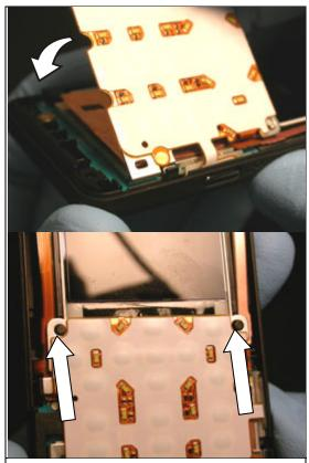
Insert the camera switch portion of the dome foil assembly into place between the circuit board and camera key.
