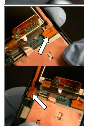
Fold the copper portion of the heat spreader down onto the circuit board's shield can. Make sure the shield can's two prongs go through the heat spreader.
