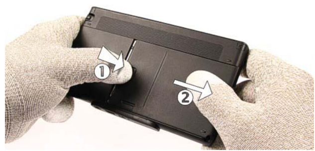
4.) Push down the Battery Cover Release Button and remove the Battery Cover. Always remove the battery before continuing disassembly.
