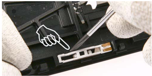
22.) Now, unlock the other side of the Antenna Assy .
