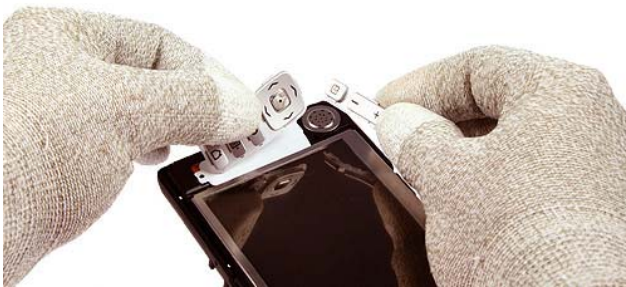
11.) Remove the Keymat Front and the Keymat Top. Display Module needs to be supported all the time when turning over the device!
