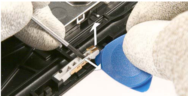
21.) Unlock the first snap. Push the Antenna Assy with a slotted screwdriver and lift it using the SRT-6 as a lever.
