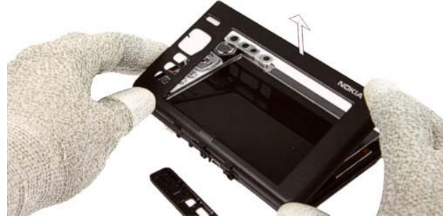
10.) Remove the A-Cover Assy by twisting it from the Fastening Cover.
