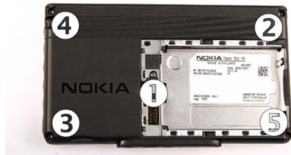
8.) Unscrew the five, Torx Plus® size 6 screws in the shown order. For assembly, use the reverse order and a Torx Plus® size 6 driver with a torque setting of 30Ncm.
