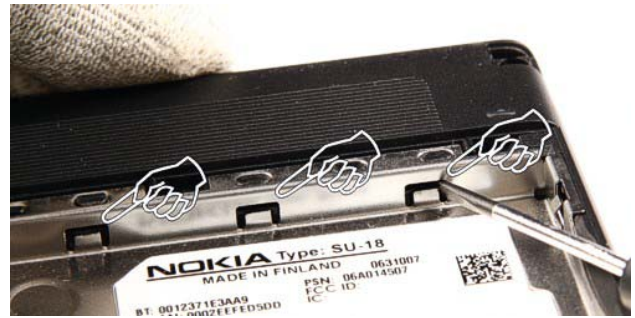
12.) Release the clips of the Battery Holder carefully. Note! It is not allowed to bend the Battery Holder Metals.
