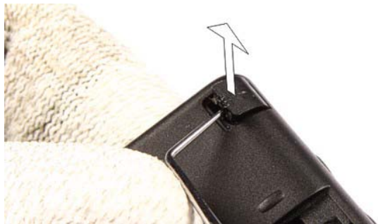
7.) Remove the Screw Covers by using the dental tool. Always use new Screw Covers when reassembling the device.
