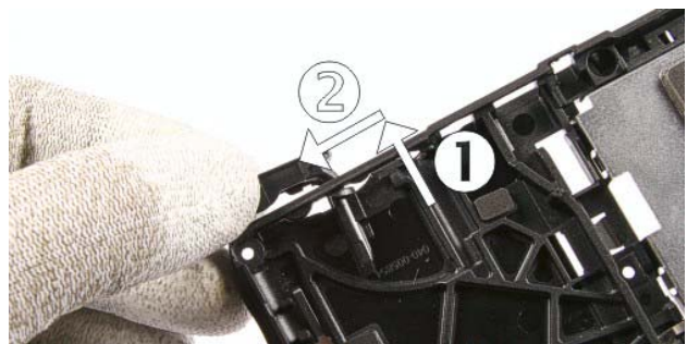
24.) Remove the MMC Cover by pushing it out and position it in the middle of its guidance.
