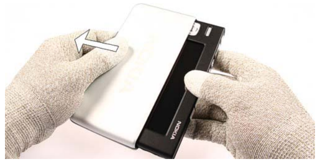
2.) Remove the C-Cover Assy.
